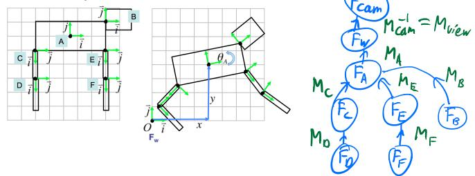
(b) (2 points) Give an algebraic expression for the composite transformation that would be used when drawing a point  $P_D$ , as defined in frame  $F_D$ .i.e., it should transform point  $P_D$  to the camera coordinate frame,  $F_{cam}$ . Your answer should be expressed as a product of the matrices used to label your scene graph.
