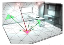
Radiosity: A ray of light that hits a surface is reflected by multiple diffuse rays, which can themselves illuminate other surfaces. Surfaces are subdivided to increase accuracy of the solution.
