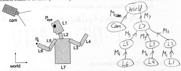
(b) (2 points) Give an expression for the composite transformation that would be used when drawing point  $P_6$ , as defined in frame  $F_6$  for link L6. i.e., it should transform point  $P_6$  to the camera coordinate frame. Your answer should be expressed as a product of the matrices used to label your scene graph.
