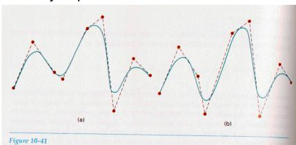
Local modification of a B-spline curve. Changing one of the control points in (a) produces curve (b), which is modified only in the neighborhood of the altered control point.
