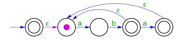
Key idea: Add ε-edges from each accepting state back to the initial state. Each time the NFA takes one of these edges, it has recognized a string from {ab, aba}. Thus, the NFA recognizes a sequence of such strings.
