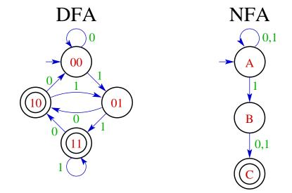
The DFA has states to keep track of the last two symbols read. State xy means that x was the next to the last symbol read, and y was the last symbol read. For example, state 10 means that the last symbol read was a 0 and the next to the last symbol read was a 1 (hence state 10 is accepting).
