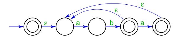
Key idea: Add ε-edges from each accepting state back to the initial state. Each time the NFA takes one of these edges, it has recognized a string from {ab, aba}. Thus, the NFA recognizes a sequence of such strings.
