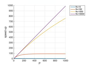
Example: Speedup of a problem where parallel work grows as N<sup>3/2</sup> and sequential work as log P.
