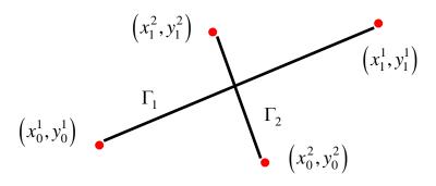
$$G_{1} = \begin{cases} x^{1}(t) = x_{0}^{1} + (x_{1}^{1} - x_{0}^{1})t \\ y^{1}(t) = y_{0}^{1} + (y_{1}^{1} - y_{0}^{1})t \end{cases} \quad t \in [0,1] \qquad G_{2} = \begin{cases} x^{2}(r) = x_{0}^{2} + (x_{1}^{2} - x_{0}^{2})r \\ y^{2}(r) = y_{0}^{2} + (y_{1}^{2} - y_{0}^{2})r \end{cases} \quad r \in [0,1]$$
