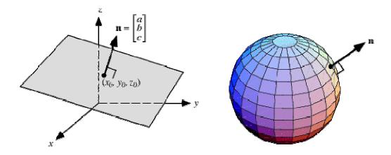
**Normal:** unit vector perpendicular to surface **Unit** vector – vector of length 1
