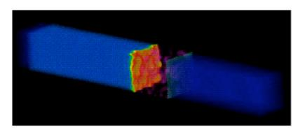
shockwave visualization: simulation with Navier-Stokes PDEs
