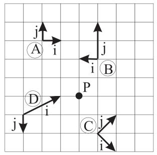
Specify the coordinates of point P with respect to coordinate frames A, B, C, and D.
