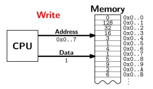
Computer memory is an array. Every bit has a physical location.
